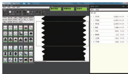
Immediate frame selection measurement (Function Area → Image Area → Data Area)
